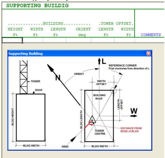
The new table configuration allows defining building parameters only ones in the Default Loading Condition. Distance from building edge to a tower will be automatically calculated for each loading condition depending on the wind azimuth.
